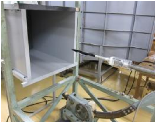
Fig.1 0.6m × 0.6m blow-down wind tunnel in University of Tokyo
