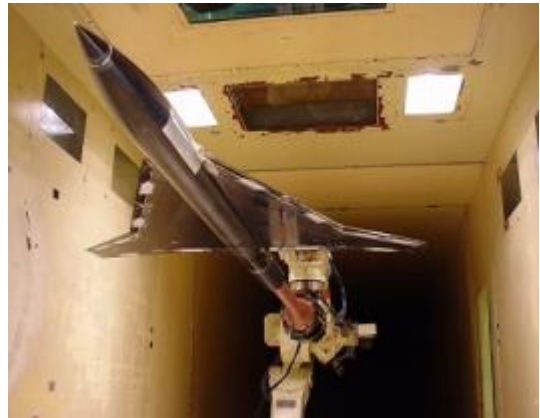
Fig.2 2m × 2m low speed wind-tunnel in JAXA
