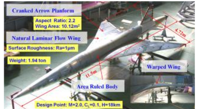
Fig. 2. NEXST-1 with aerodynamic design concepts
