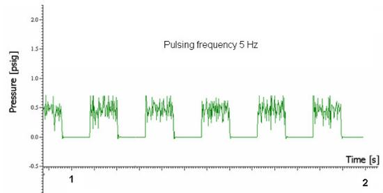
Fig 4: Typical measured jet output dynamic pressure trace.
