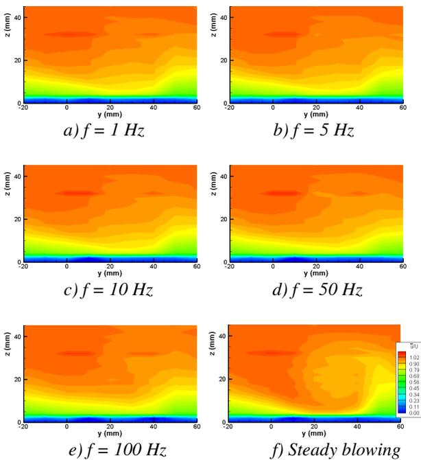
Fig 12: Contours of Streamwise Component of Velocity.  $VR=3.2$ ,  $x = 400\text{mm}$ .
