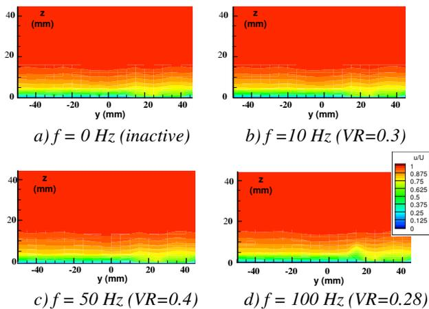
Fig 14: Contours of Streamwise Component of Velocity. Synthetic Jet,  $U = 25\text{m/s}$ ,  $x = 100\text{mm}$ .
