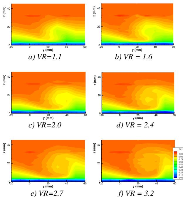
Fig 8: Contours of Streamwise Component of Velocity. Steady Blowing,  $x = 400mm$ .
