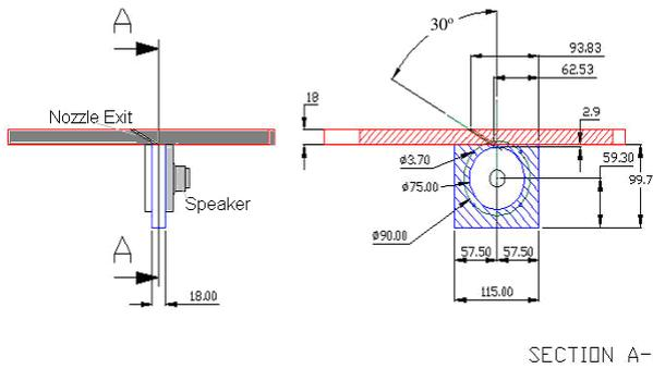
Fig 5: The acoustic synthetic jet actuator design.
