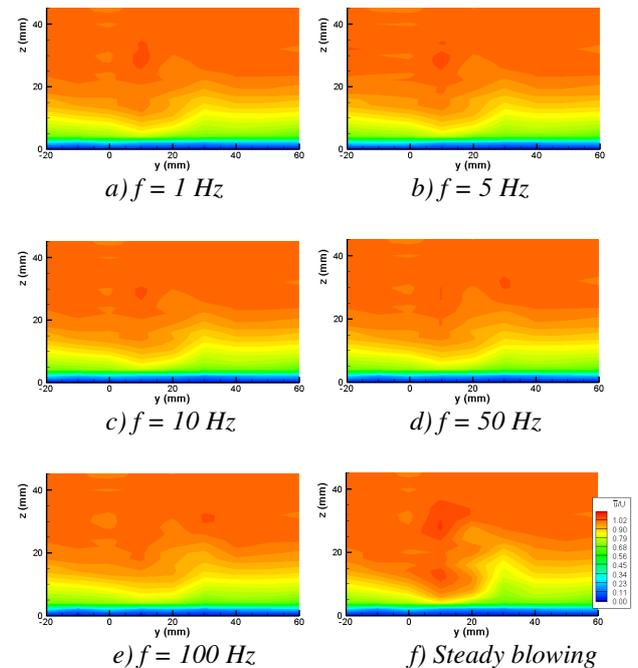
Fig 11: Contours of Streamwise Component of Velocity.  $VR=3.2$ ,  $x = 100\text{mm}$ .
