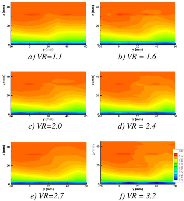
Fig 10: Contours of Streamwise Component of Velocity. Pulsed Blowing at 100Hz,  $x = 400\text{mm}$ .
