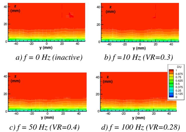
Fig 13: Contours of Streamwise Component of Velocity. Synthetic Jet,  $U = 25\text{m/s}$ ,  $x = 50\text{mm}$ .
