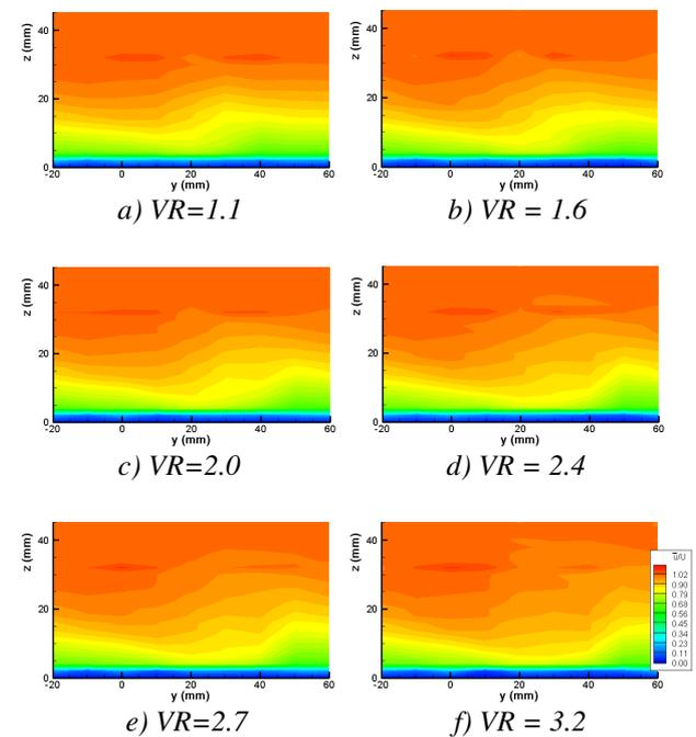
Fig 9: Contours of Streamwise Component of Velocity. Pulsed Blowing at 1Hz.,  $x = 400mm$ .
