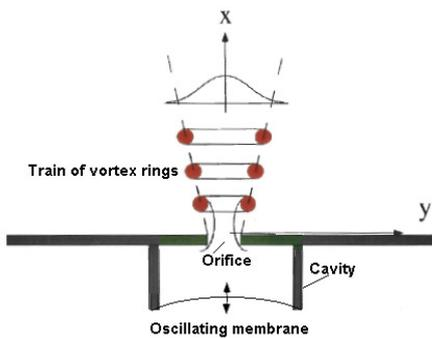
Fig 2: Schematic of acoustic synthetic jet flow.
