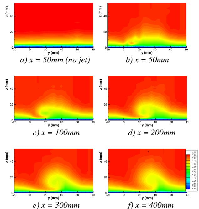
Fig 7: Contours of Streamwise Component of Velocity. Steady Blowing.  $U=30$ m/s,  $VR=2.0$ .
