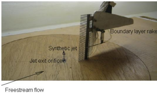
Fig 3: Experimental arrangement of boundary layer rake.
