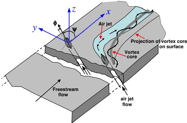
Fig 1: Schematic of steady air jet flow / streamwise vortex generation.
