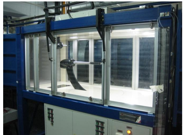
Fig. 4 Closed-circuit wind-tunnel test section with sting balance
