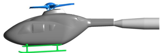
Fig. 6. Geometry used for numerical simulation of the W/T model flow.
