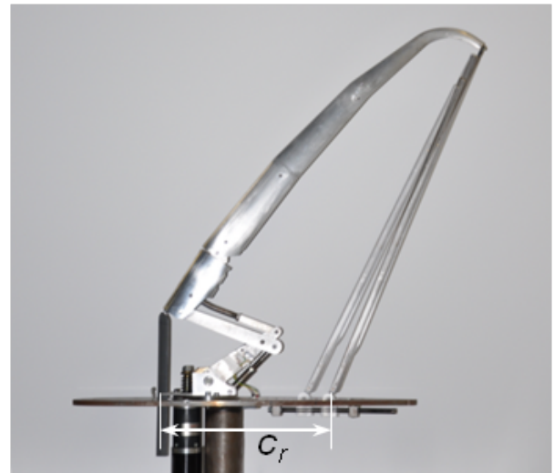
Fig. 3 Illustration showing the movable trailing-edge of the wind tunnel model (here in the swept-back planform configuration). The root chord length c_r can be varied between 0.24 and 0.27 m.
