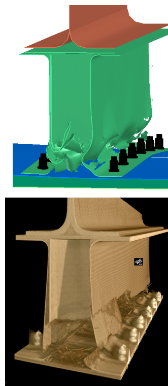
Fig. 13. Comparison of failure modes (DY1): numerical model (top) and HRCT scan (bottom)
