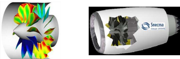
Counter rotating fan with 10 + 14 blades
