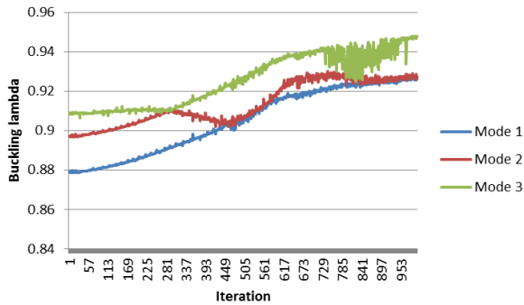
Figure 14: Convergence of mode 1 and 2 for the second local optimization. Initially a larger deviation between the modes is present.
