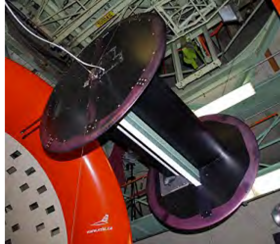
Fig. 1 Model equipped with the airbrake in the test section
