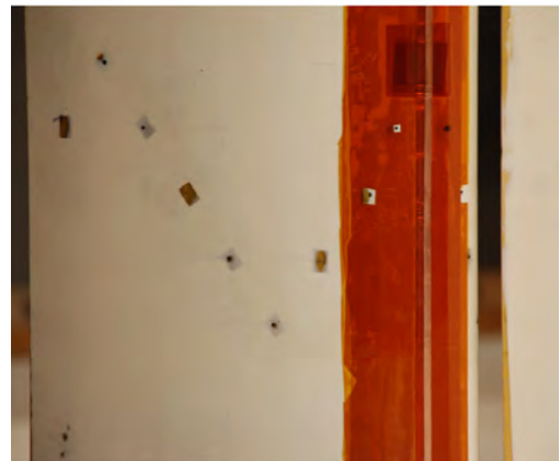
Fig. 20 Standard DBD actuator positioned close to the LE of the flap. At the dark rectangular area multiple layers of dielectric were placed to prevent discharge with the metal orifice.
