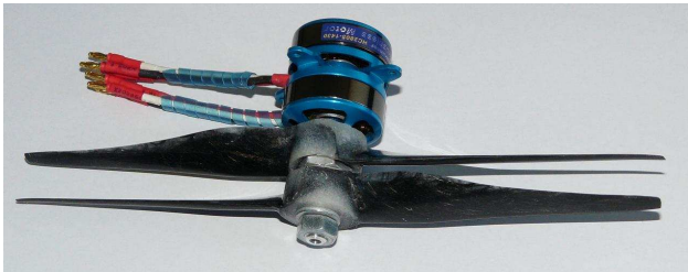
Fig. 4 Set of counter rotating motor with the designed propellers.
