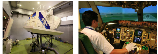
Fig. 2 Outside and inside of ANA's Boeing 767-300 simulator
