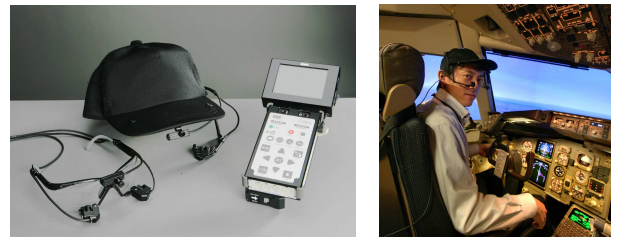
Fig. 3 NAC's EMR-9 eye-mark recorder ( left ; photo by NAC, reproduced with permission) and the pilot wearing it ( right )
