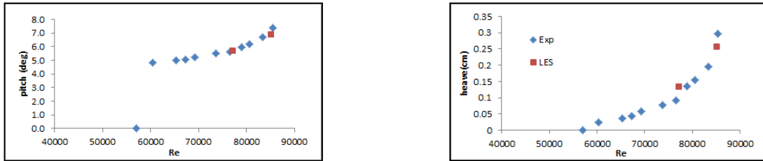
Figure 5. Pitch angle and heave response of the 2DOF pitch-heave NACA 0012 airfoil as a function of Reynolds number.
