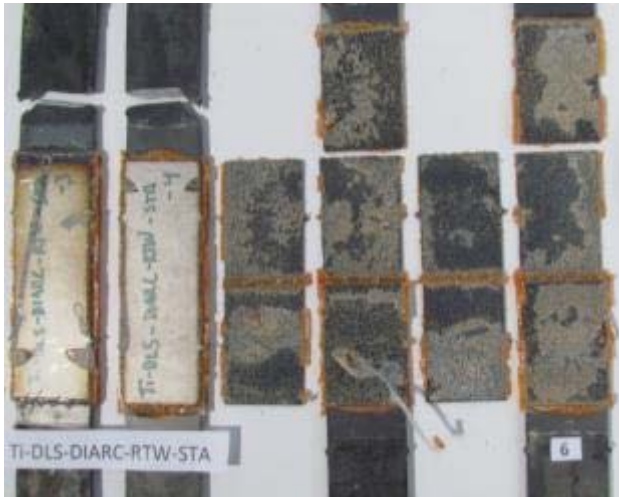
Fig. 7. Typical failure modes of titanium double lap shear specimens with the DIARC treatment. Two specimens had adherend failure modes while two specimens failed cohesively in the bondline.
