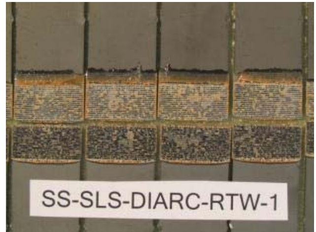
Fig. 2. Typical cohesive failure mode of stainless steel AISI 304 (SS) single lap shear specimens with DIARC treatment and FM300-2 adhesive film tested at room temperature as wet (RTW).
