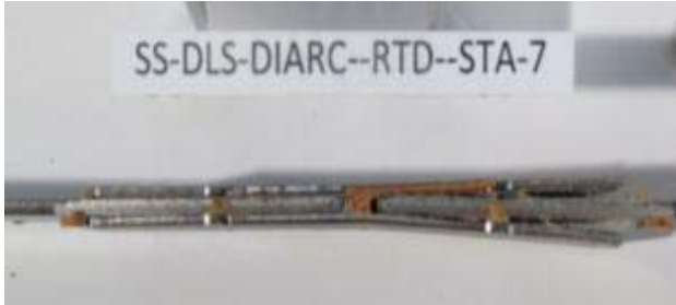
Fig. 6. Typical plastic deformation and cohesive failure mode in the doubler ends of stainless steel AISI 304 (SS) double lap shear specimens.
