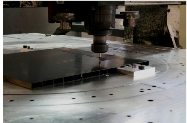
Fig. 12. Photograph showing a slot in the first 1 x 10 array being cut by the CNC router.
