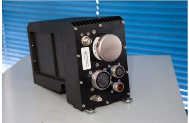
FIG. 10. BAE SYSTEMS AUSTRALIA'S FLIGHT CONTROL COMPUTER (FCC) USED FOR VEHICLE MANAGEMENT OF KINGFISHER 2 PLATFORM.
