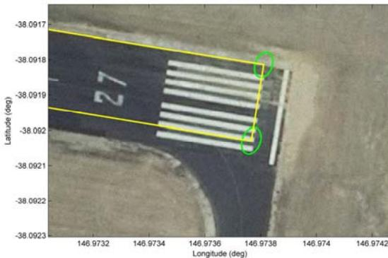
FIG. 34. RUNWAY POSITION SOLUTION DURING FLIGHT TEST (27 RUNWAY END).
