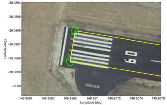
FIG. 25. RUNWAY POSITIONING SOLUTION FOR SIMULATED NORMAL FLIGHT EXTENTS (09 RUNWAY END).
