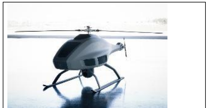
Fig. 1 The autonomous helicopter Skeldar V200
