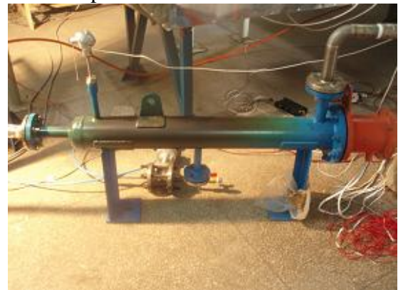
Fig.3. Electrical Heater of Air
