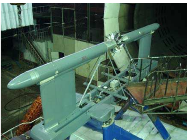
Fig. 4. VP-107 Test Vehicle in TsAGI Low Speed T-104 Wind Tunnel (DREAM project)
