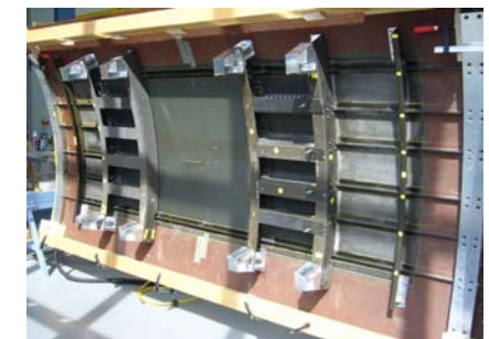
Fig. 21: ALCAS Door Surround test panel
