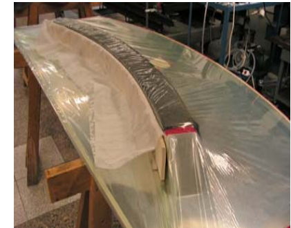
Fig. 12: Bladder forming, frame preform
