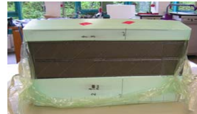
Fig. 15: PMI foam cores, Intercostal preform
