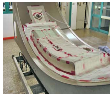
Fig. 14: Manufacturing set-up on primary mould
