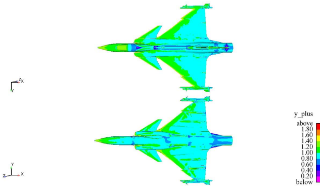
Fig. 5. y^+ distribution at supersonic speed. The common range is 0.8 < y^+ < 1.5 . Only at the leading edges y^+ exceeds 1.5, though below 1.8 on the main wing and below 2 on the canard leading edge.
