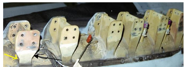
Fig. 1 A view of starboard attachment stubs after removal of vertical tail. The Y598 stub is marked with an arrow (aft is to the left).
