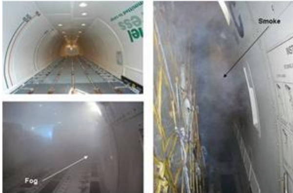
Figure 4: Fog vs. smoke environment in cargo compartments
