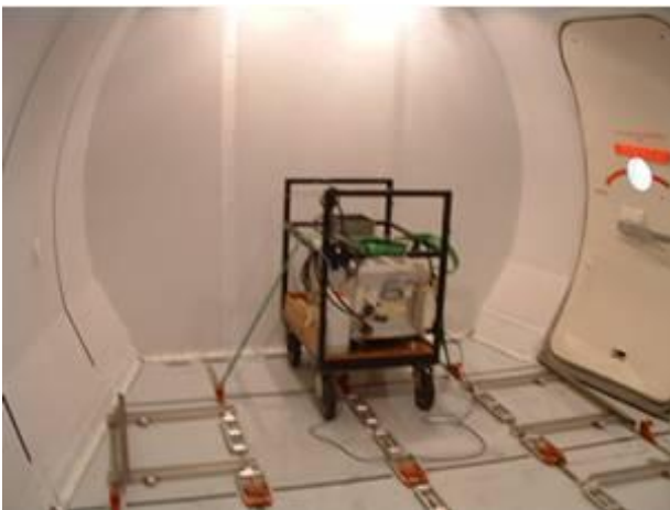
Figure 22: Smoldering smoke generator
