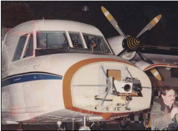
Fig. 4. Example of sensor installation.
