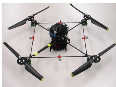
Fig. 5 Quadrotor vehicle equipped with reference markers.
