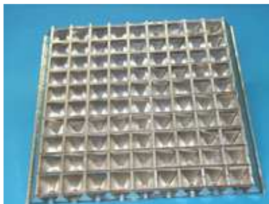
Fig. 4: The so-called ULSAP resonators
