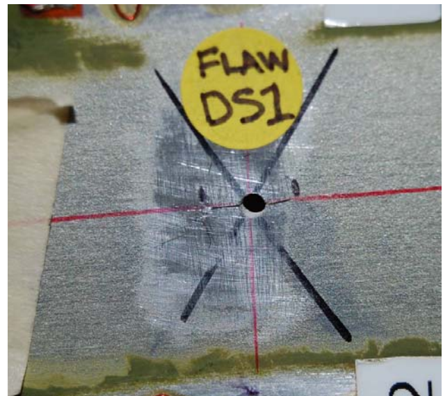
Fig. 11. ST-013 flaw initial installation
