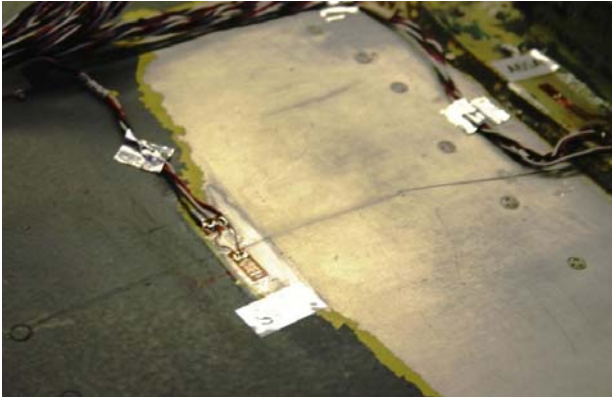
Fig. 19. ST-016 flaw crack 2 after limit load test #1
