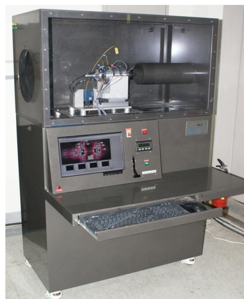
Fig. 2 Complete Test Setup of I-Jet 130 Engine
