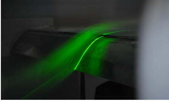
Fig. 21. Laser visualization - Flap 45, with AFC
