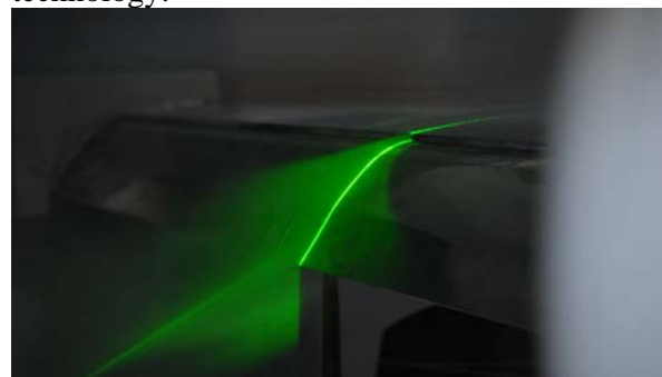
Fig. 20. Laser visualization - Flap 45, no AFC
