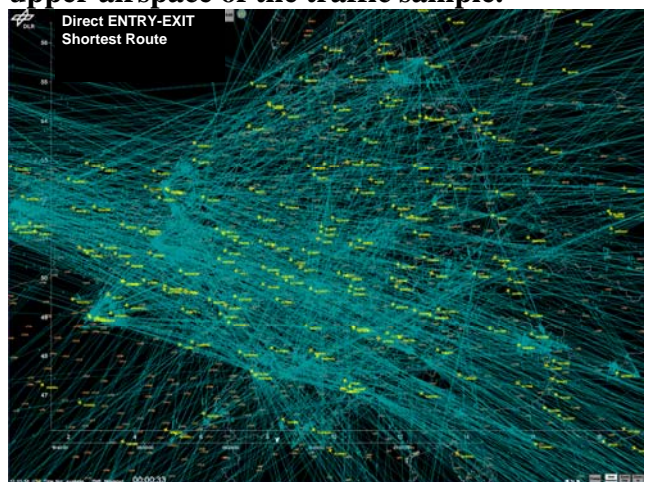
Figure 6. The same traffic sample as in Figure 5. However, every aircraft is flying the shortest path. It can be seen clearly that there is a far better use of the existing airspace.
