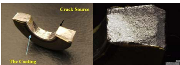
Fig. 6. Fracture surfaces of lap/butt joints
