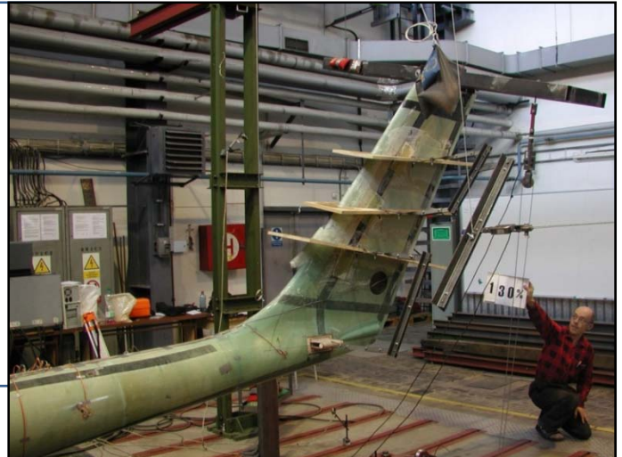
Fig. 2.3 – Comparison of Finite Element analysis (MSC PATRAN/ NASTRAN) and structural test of composite fuselage
