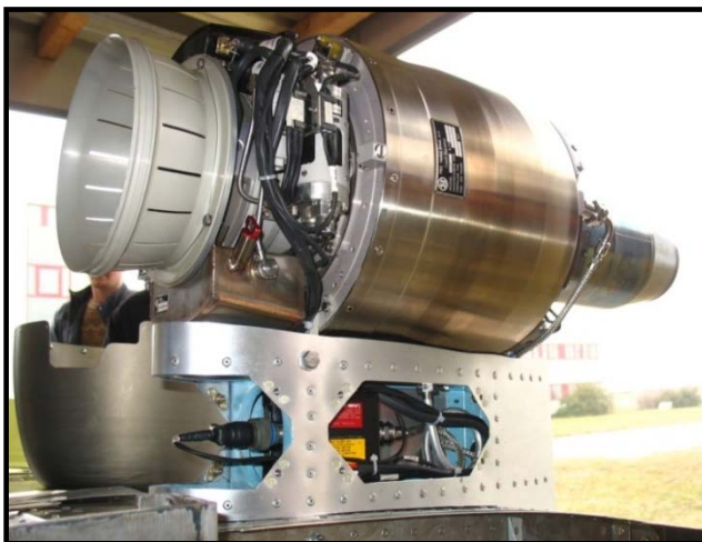
Fig. 2.4 – TJ100M installed on the wing centre section of VUT 001 Marabu
