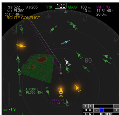
Figure 1. A screenshot of CSD displaying radar weather, traffics, and conflict alerts
