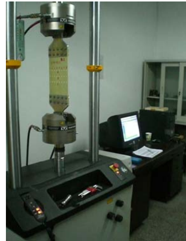
Fig. 3. Specimen Gripped in Fatigue Machine
