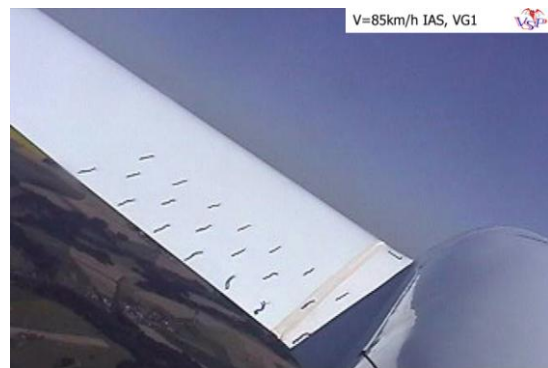
Fig. 19b. TST10a sailplane, wing root tuft visualization, V = 85 km/h IAS, passive-flow control: vane-type VG, x_{VG}/c = 0.45
