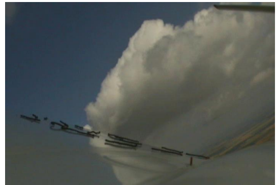
Fig. 16b. VSO10C sailplane, wing root tuft visualization, V = 70 km/h IAS, bank angle 30deg, stalled flow
