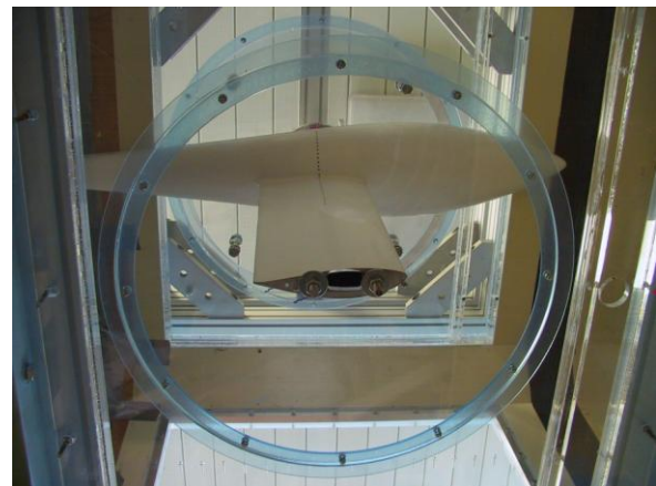
Fig. 7. T10 test case geometry in the 865 \times 485 \text{mm}^2 wind-tunnel IT AS CR
