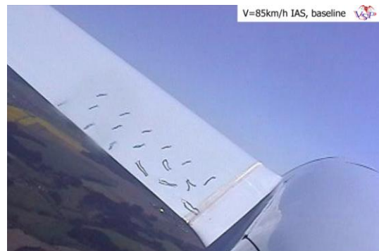
Fig. 19a. TST10a sailplane, wing root tuft visualization, V = 85 km/h IAS, uncontrolled case
