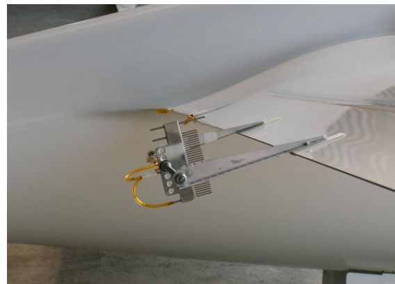
Fig. 9. Installation of pressure rake downstream the wing trailing edge
