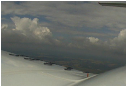
Fig. 16a. VSO10C sailplane, wing root tuft visualization, V = 140 km/h IAS, attached flow
