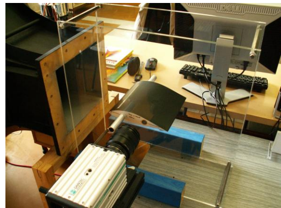
Fig. 6. Blow-down rig 250 \times 250 \text{mm}^2 IT AS CR, TR PIV setup
