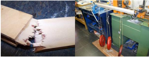
Fig. 10. Loading tests until crash
