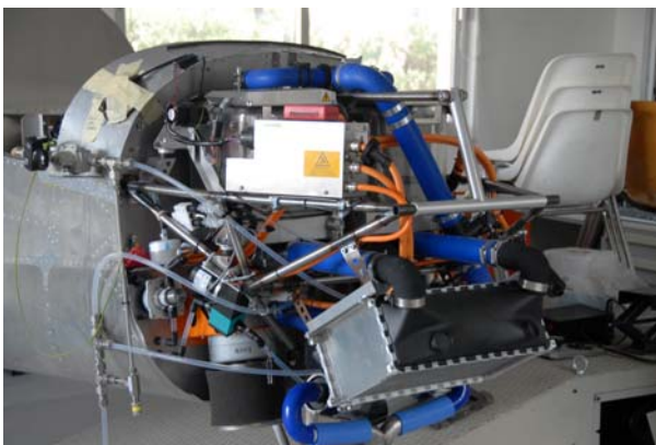
Fig. 7. Fuel cell system assembled in the mock-up fuselage
