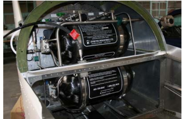
Fig. 10. Hydrogen storage system.
