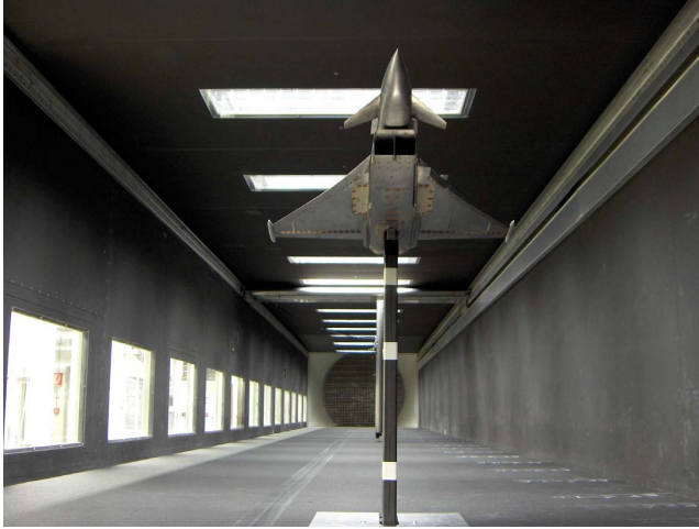
Fig. 1 Delta-canard configuration mounted in the test section of wind tunnel C
