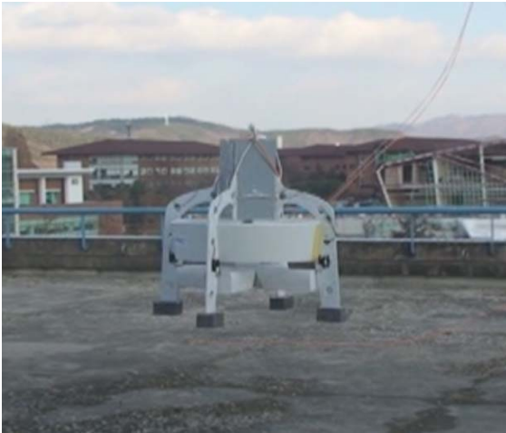
Fig. 14. Flight Test of a Shrouded Propeller
