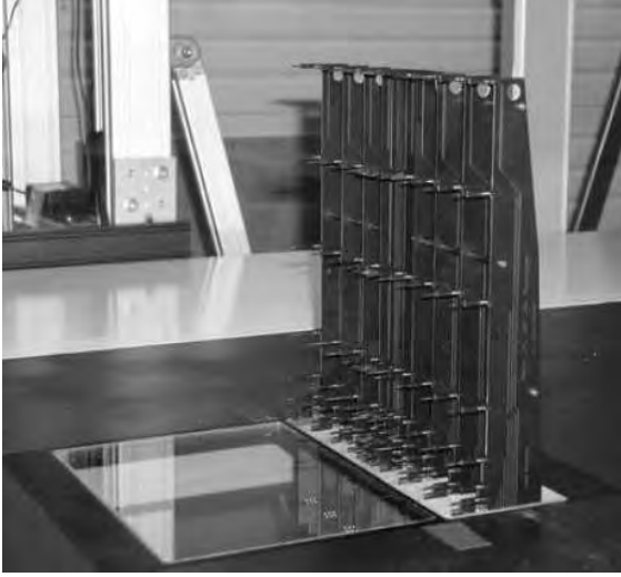
Fig. 3 Hot-wire rake in place in the LML wind tunnel.
