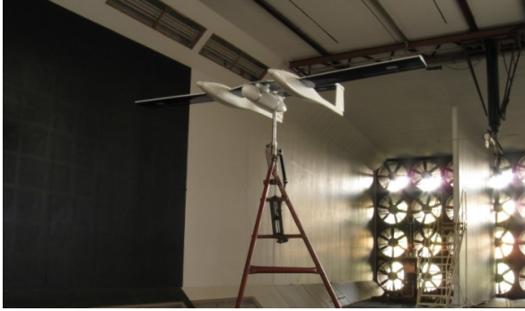
Fig. 5: The Modular UAV baseline configuration in the CSIR 7M wind tunnel
