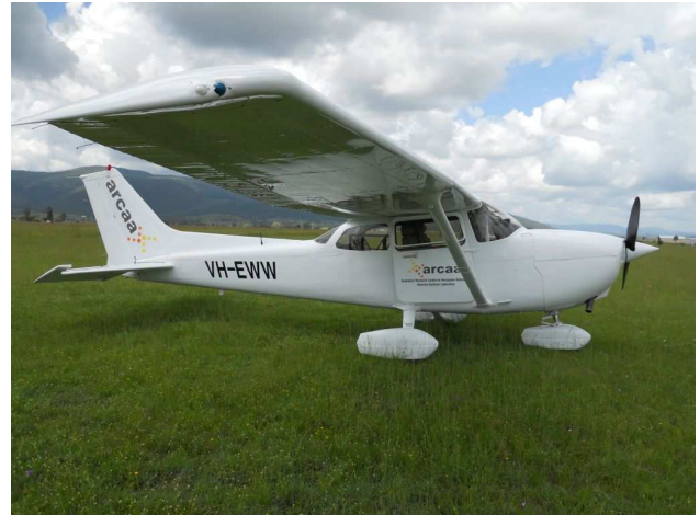
Fig 4. The Airborne Systems Laboratory (ASL) is a Cessna 172R.
