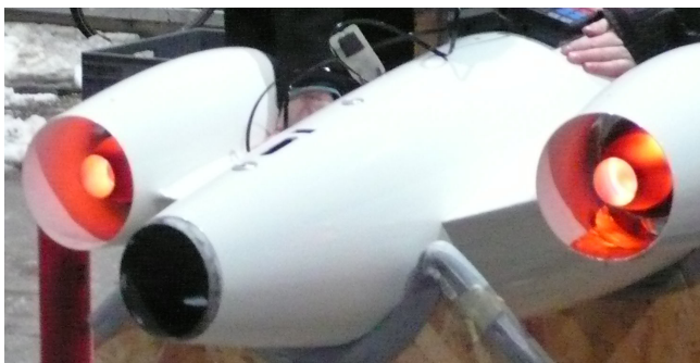
Fig. 9 Engine full throttle test and thrust measurement (440N) (performed in UST)
