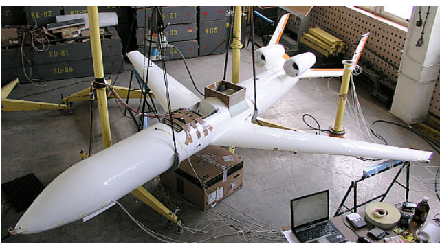
Fig. 7 Ground Vibration Tests carried out in the IoA
