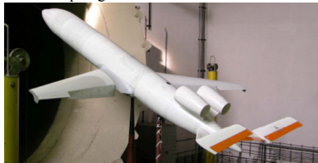
Fig. 6 IEP 15 Model in Wind Tunnel T3, IoA
