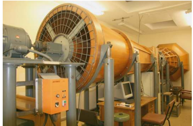
Figure 3.5 Calibration Wind Tunnel
