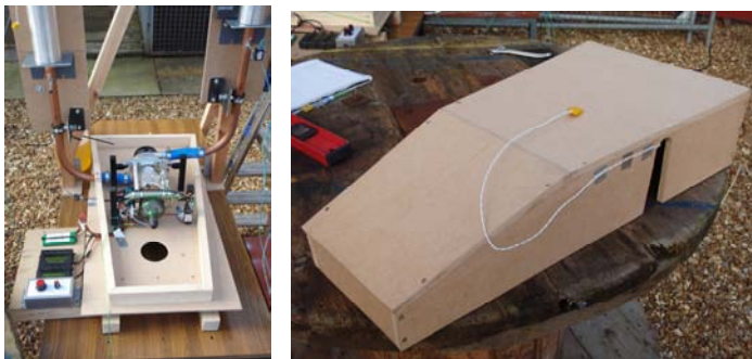
Figure 11: The APU enclosed in the dummy Demon nose bay
