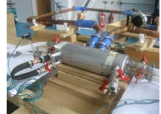
Figure 13: The Valve Block, core of the Pneumatic Power Control System of the Demon UAV.
