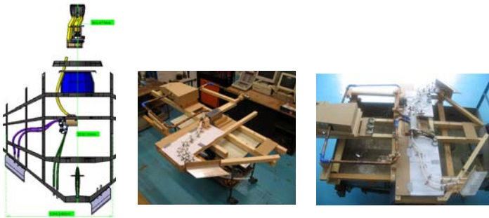
Figure 11: The Ironbird for the Demon Pneumatic Power System. From left to right: design phase, Mk1 and Mk2.
