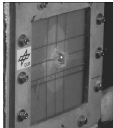
Fig. 4. Shot on a demonstrator plate made of GFRP and Tegriss as “Catching Membrane” (300x300x5,1mm)
