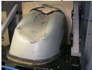
BP test shot and U-frame post test damage
