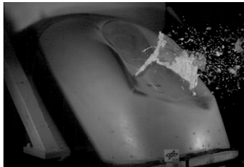
BP test shot and U-frame post test damage
