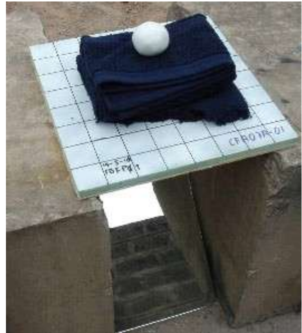
Fig. 5. Arrangement for shock-holing tests on composite panels
