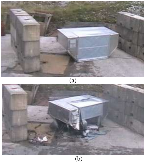
Fig. 4. Un-Strengthened ULD Blast test (a) Pre-Test (b) Post Test
