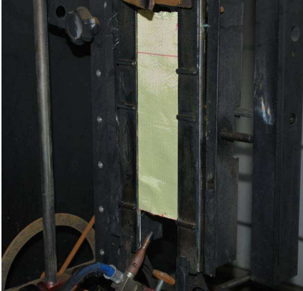
Fig.5. Flame test rig for fire testing of textiles available at STFI
