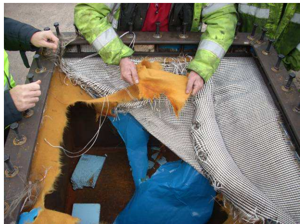
Fig. 7. Result of preliminary test of fabric layer showing tearing of the material
