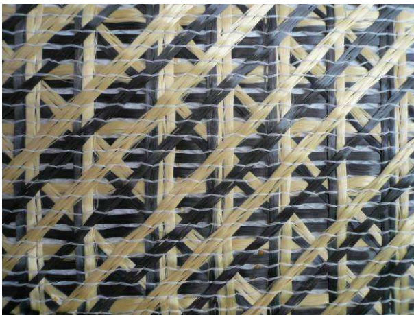
Fig.2. Blastworthy hybrid textile structures: plain wave hybrid structure made of carbon and dyneema fibres (above) and multiaxial structures from carbon and aramid fibres (below)
