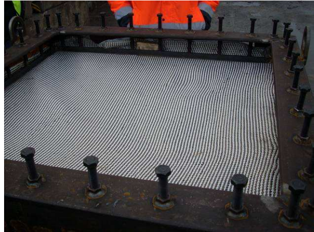
Fig. 6. Test box for the evaluation of the performance of textile layers against the Quasi Static Pressure generated by an explosive charge placed inside the box
