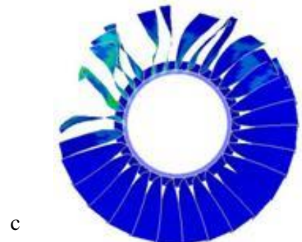
Fig. 18. Graph and illustrations showing the energy absorbed by the blade along three angles studied at 500mm of the span. Post impacts at a)75 0 b)60 0 and c)45 0 are shown
