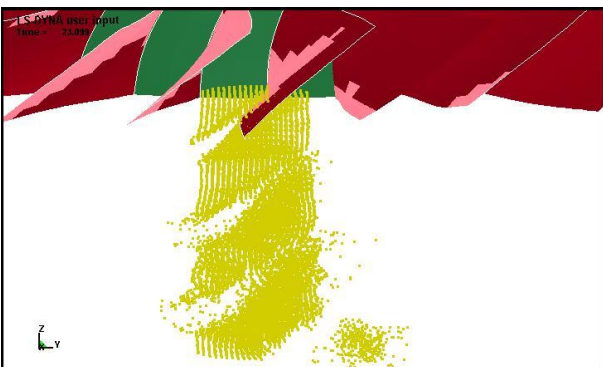
Fig. 20. Post-Impact of the bird after it struck the blades at approximately zero angle of attack.
